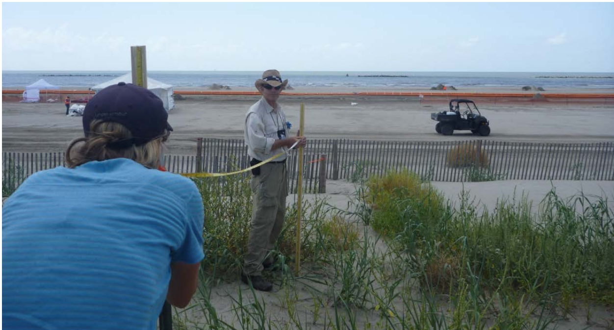
Figure 1. Beach profiling using the rod-and-horizon method.
