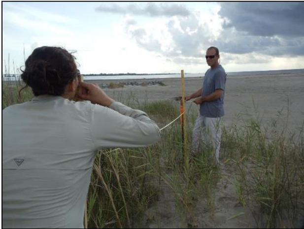
The horizon must be visible to conduct the Emery Method. If fog or rain obscures the sea/sky horizon, the survey cannot be done on that day.
